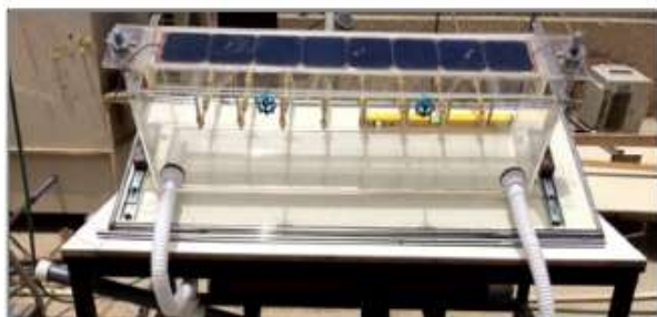
Jet Impingement Test Rig Installed on Site
