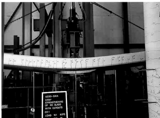
(a) 3-point flexural slab test setup
