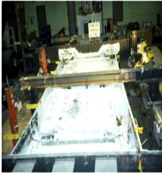
a. Innovative Composite Shear Wall
