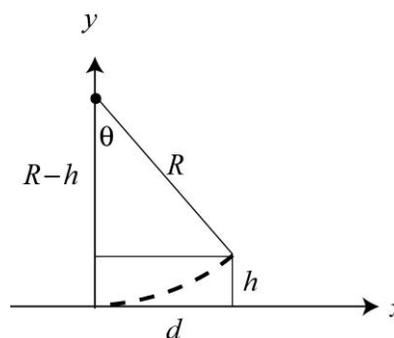
Substituting  $R = 6.72 \text{ m}$  and  $d = 0.20 \text{ m}$  into the expression, we obtain  $h = 0.0030 \text{ m}$ .
