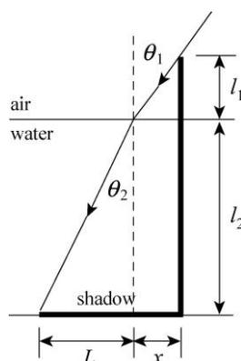
Here  $\theta_1 = 90^\circ - \theta = 90^\circ - 55^\circ = 35^\circ$ ,  $\ell_1 = 0.50$  m, and  $\ell_2 = 1.50$  m. The length of the shadow is  $d = x + L$ .
