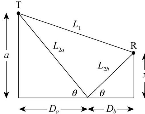
The right triangle on the left, formed by the vertical line from the water to the transmitter T, the ray incident on the water, and the water line, gives  $D_a = a / \tan \theta$ . The right triangle on the right, formed by the vertical line from the water to the receiver R, the reflected ray, and the water line leads to  $D_b = x / \tan \theta$ . Since  $D_a + D_b = D$ ,
