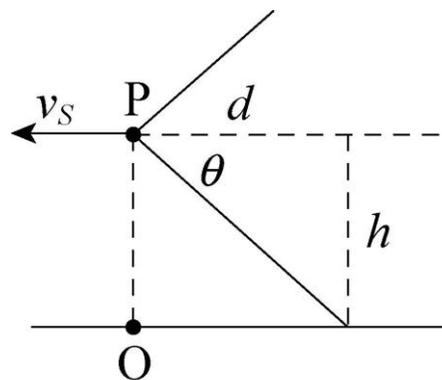
The cone angle is related to  $h$  and  $d$  by  $\tan \theta = h/d$ , so  $d = h/\tan \theta$ . The shock wave reaches O in the time the plane takes to fly the distance  $d$ .
