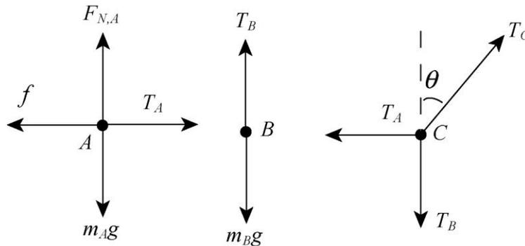
The tensions in the three strings are denoted as  $T_A$ ,  $T_B$  and  $T_C$ . Analyzing forces at C, the conditions for static equilibrium are
