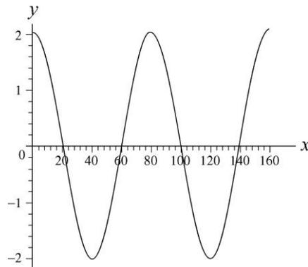
(c) The wave can be written as  $y(x,t) = y_m \sin(kx + \omega t)$ , where  $v = \omega/k$  is the speed of propagation. From the problem statement, we see that  $\omega = 2\pi/0.40 = 5\pi$  rad/s and  $k = 2\pi/80 = \pi/40$  rad/cm. This yields  $v = 2.0 \times 10^2$  cm/s = 2.0 m/s.
