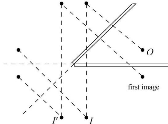
(c) For  $\theta = 60^\circ$ , we have two images in the second mirror caused by the object and its “first” image, and from these one can construct two new images  $I$  and  $I'$  behind the first mirror plane. The images  $I$  and  $I'$  are each other’s “twins” in the sense that they are each other’s reflections about the extension of the second mirror plane; there are no further images. Summarizing, we find  $1 + 2 + 2 = 5$  images in this case.
