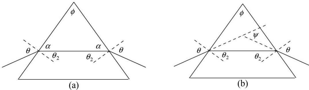
**ANALYZE** Next, examine diagram (b) and consider the triangle formed by the two normals and the ray in the interior. One can show that  $\psi$  is given by
