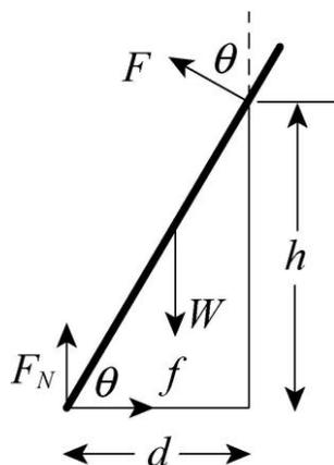
Its magnitude is designated  $F$ .  $W$  is the force of gravity; this force acts at the center of the plank, a distance  $L/2$  from the point where the plank touches the floor.  $F_N$  is the normal force of the floor and  $f$  is the force of friction. The distance from the foot of the plank to the wall is denoted by  $d$ . This quantity is not given directly but it can be computed using  $d = h/\tan\theta$ .
