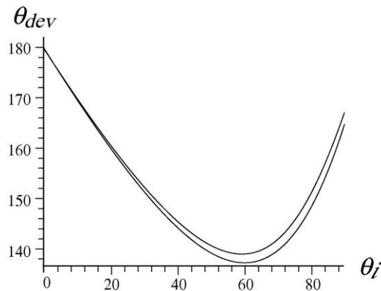
(c) We can expand the graph and try to estimate the minimum, or search for it with a more sophisticated numerical procedure. We find that the  $\theta_{\text{dev}}$  minimum for red light is  $137.63^\circ \approx 137.6^\circ$ , and this occurs at  $\theta_i = 59.52^\circ$ .
