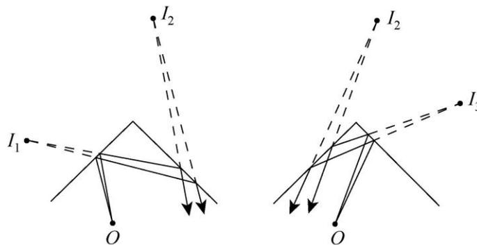
We may consider  $I_2$  to be the image of  $I_1$  formed by the right-hand mirror, extended.  $I_2$  is the same distance behind the line of the right-hand mirror as  $I_1$  is in front, and it is on the line that is perpendicular to the line of the mirror. The diagram on the right shows image  $I_3$ , formed by reflections from the right-hand mirror. It is the same distance behind the mirror as the object is in front, and lies on the line perpendicular to the mirror and
