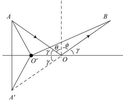
Since  $\theta + \gamma = \phi + \gamma = \pi/2$ , we readily see that  $\theta = \phi$ , i.e., the angle of incidence is equal to the angle of reflection. To show that  $AOB$  is the shortest path, consider an incident ray  $AO'$  with a reflected ray  $O'B$ , where the angle of incidence is not equal to the angle of reflection. From the figure, we have
