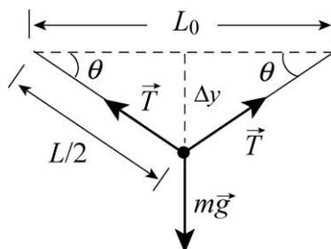
The condition for equilibrium is  $mg = 2T \sin \theta$ , where  $m$  is the mass of the insect and  $T = A(\text{stress})$ . Since the volume of the thread remains constant as it is being stretched, we have  $V = A_0 L_0 = AL$ , or  $A = A_0(L_0 / L) = A_0 / 3$ . The vertical distance  $\Delta y$  is
