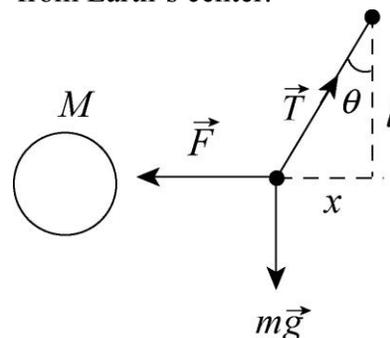
The force between the “spherical” mountain and the plumb line is  $F = GMm/r^2$ . Suppose at equilibrium the line makes an angle  $\theta$  with the vertical and the net force acting on the line is zero. Therefore,
