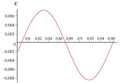
This is close enough to a regular sine wave cycle that we can estimate its period ( $T = 0.18$  s, so  $\omega = 35$  rad/s) and its amplitude ( $y_m = 0.008$  m).
