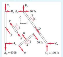
Alternatively we could have returned to the free-body diagram of the frame as a whole and found  $C_x$ .
