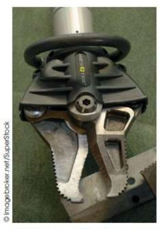
This "jaws-of-life" machine is used by rescuers to pry apart wreckage.
