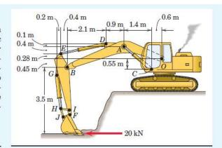
**Solution.** (a) We begin by constructing a free-body diagram of the entire arm assembly. Note that we include only the dimensions necessary for this portion of the problem—details of the cylinders *DE* and *GH* are unnecessary at this time.
