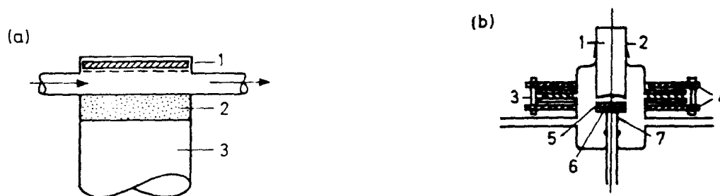
Fig. 3.40. (a) The principle of measurement of adsorbed radioactivity. 1 --- catalyst or electrode; 2 --- scintillator; 3 --- photomultiplier. Reproduced by permission of Mink et al. [3.21]. (b) High temperature chamber for the continuous monitoring of radiotracers on a catalyst surface. 1 --- GM-tube; 2 --- rubber seal; 3 --- Teflon gasket; 4 --- brass clamps; 5 --- catalyst; 6 --- heating coil; 7 --- thermocouple. After Norval and Thomson [3.35], reproduced by permission of The Chemical Society, London
