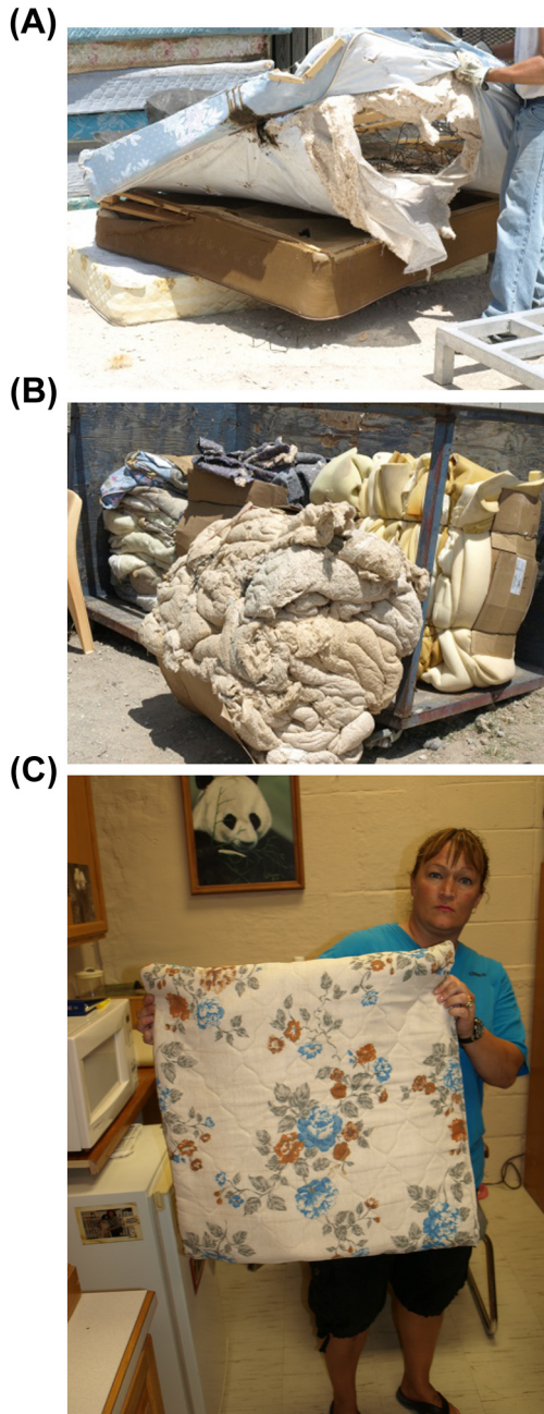
FIGURE 15.3 Mattress recycling at the Hutchinson Correctional Facility. (A) Inmates at HCF dismantle mattresses. (B) Mattress components are baled to be sold to recyclers. (C) Pet crate pads are made from recycled mattress components at the HCF. Photos courtesy of author.
