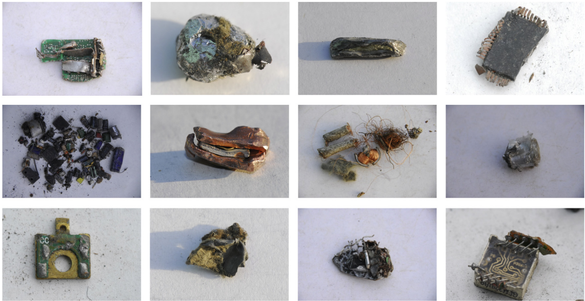
FIGURE 22.39 Particulate quality (determining recycle quality and recovery/losses) as a function of design. An impression of unliberated and multimaterial particles as found in various WEEE recyclates.
