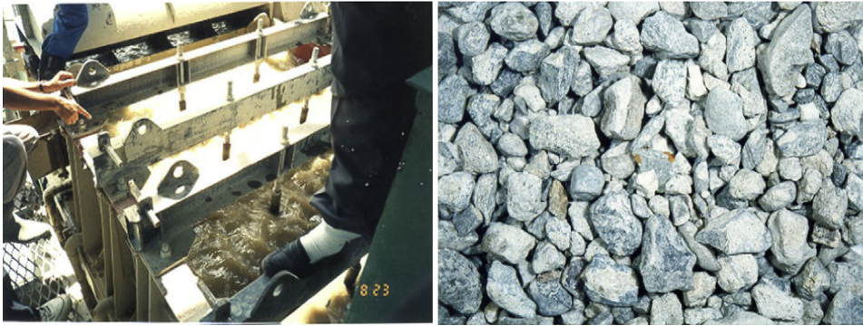
FIGURE 24.3 Gravity concentration method (Tatemastu et al., 2003).
