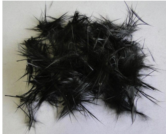
FIGURE 19.5 Recycled (through pyrolysis) carbon fibers (CFs) in discontinuous, unsized, filamentized and unstructured (fluffy) form.
