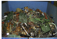
Printed Wire Boards PGMs, PMs, Sb, Ta, REs (and Fe, Al, Cu, Pb, Ni, Sn, As, Ba, Br, Bi, etc.)
