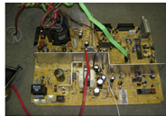
Printed Wire Boards PGMs, PMs, Sb, Ta, REs (and Fe, Al, Cu, Pb, Ni, Sn, As, Ba, Br, Bi, etc.)
