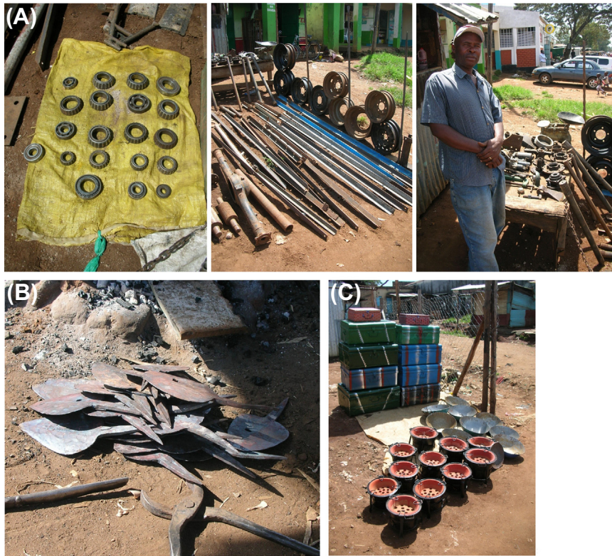
FIGURE 30.9 Examples of material reuse in Rongo Town Kenya ( Courtesy of Chris Cleaver ): (A) a scrap metal hawker; (B) small hoe blades formed from scrap metal; (C) cooking stoves and metal boxes made from scrap metal. Images © Christopher Cleaver, 2013.
