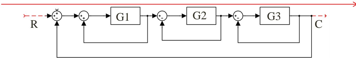
$$P_1 = G_1 G_2 G_3 ; L_1 = +G_1, L_2 = -G_2, L_3 = -G_3, L_4 = -G_1 G_2 G_3$$
