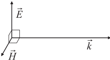
Fig. 3.3 The relative orientation of the electric and magnetic fields and the wavevector in a plane wave.
