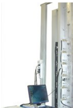
FiSER filament stretching extensional rheometer
