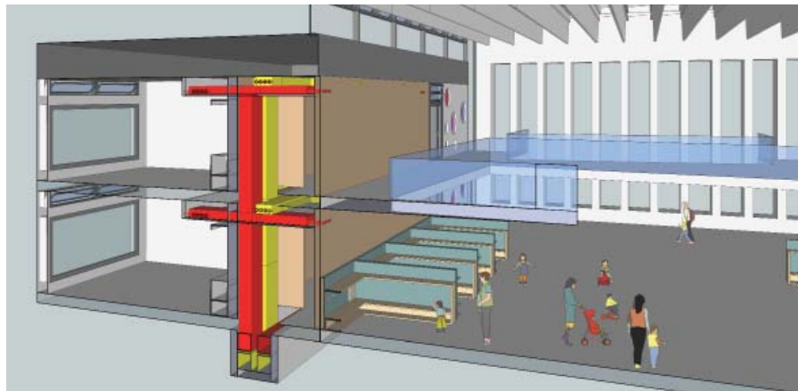
FIG. 5.12. VERTICAL SHAFTS WITH VENTILATION DUCTS.
