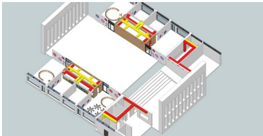
FIG. 5.13. MECHANICAL VENTILATION SCHEME ON THE GROUND FLOOR.
