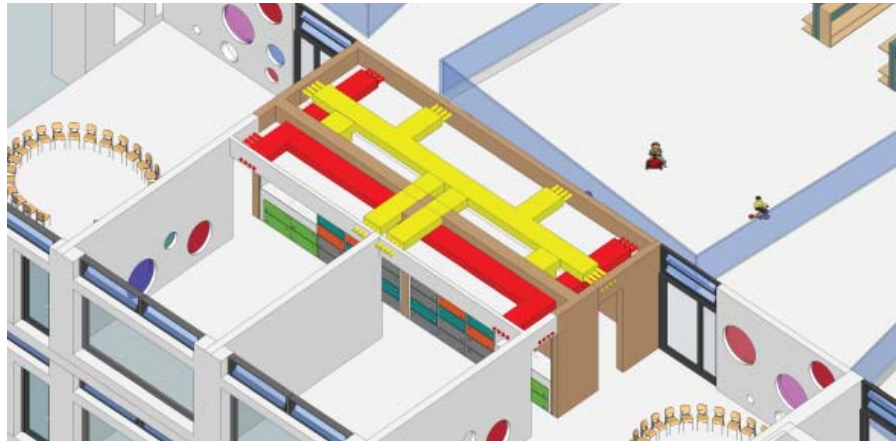
FIG. 5.11. MECHANICAL VENTILATION SCHEME IN THE CLUSTER.
