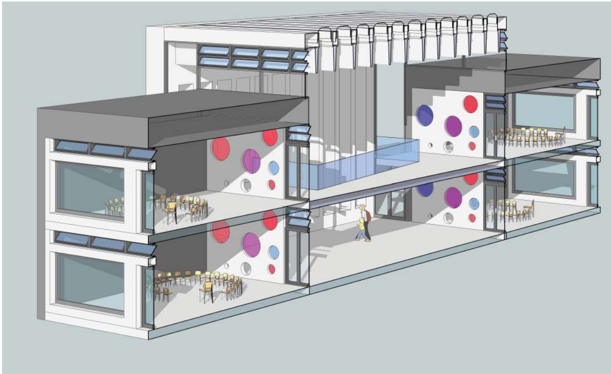
FIG. 5.18. NATURAL VENTILATION THROUGH STACK EFFECT IN ATRIUM.
