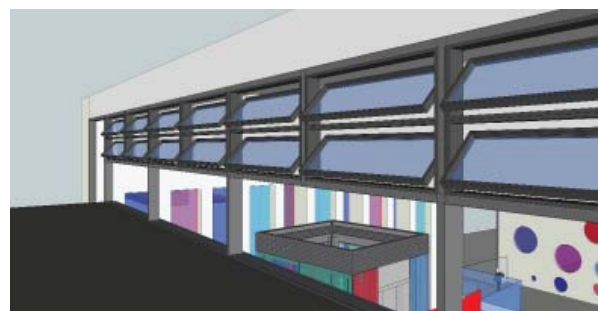
FIG. 5.17. LAMELLA IN ATRIUM'S GLAZING.
