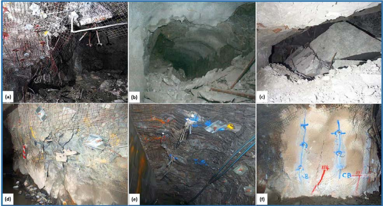
Fig. 12. Some typical failures in deep underground mines in Western Australia: (a) ground fall, (b) rockburst, (c) wedge failure, (d) blocky undercutting, (e) bulking, and (f) pillar burst.
