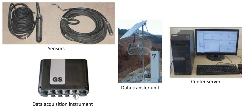
Fig. 1 The components of a microseismic monitoring system
