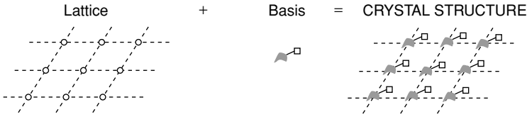
FIGURE 7.12. Schematic of a structure consisting of one point lattice and a unique basis.
