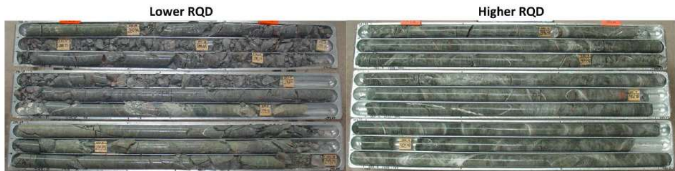
Figure 5 – Examples of core RQD
