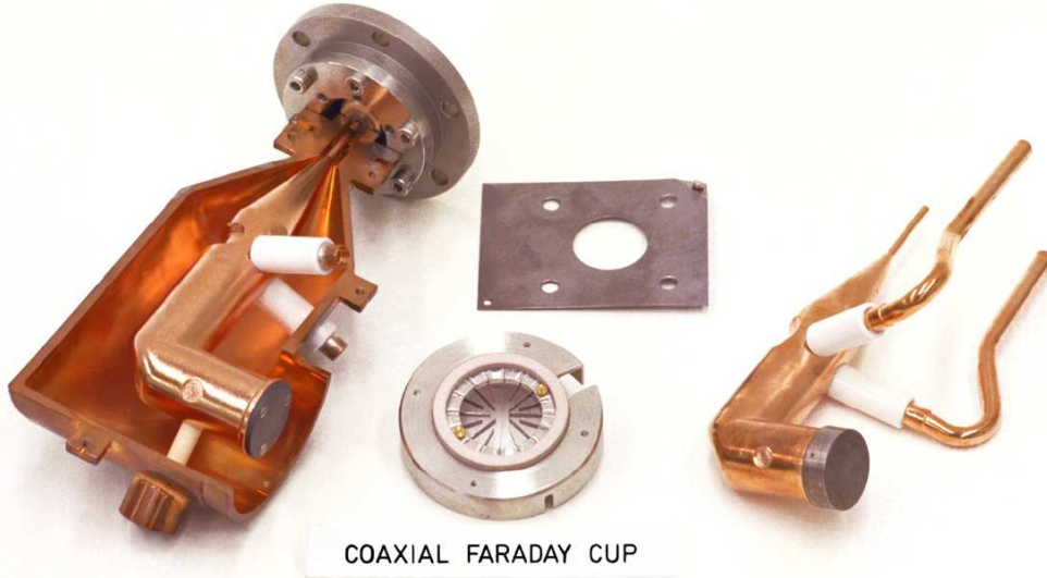
Figure 6.17: Head of a coaxial Faraday cup. The grid for shielding of the advanced field and suppression of secondary electrons is shown in the middle. The collector including the ceramic cooling water feed-through is seen on the right hand side.
