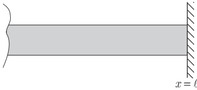
Figure 3.10. Clamped end of a beam
