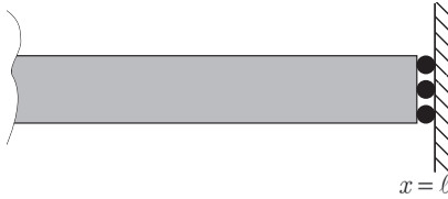
Figure 3.26. Schematic of sliding-end condition
