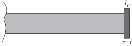
Figure 3.16. Inertially restrained end of a beam
