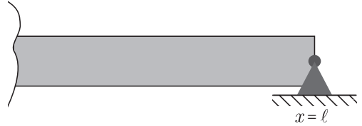
Figure 3.25. Schematic of pinned-end condition
