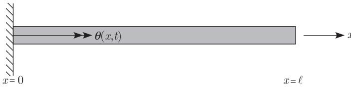
Figure 3.17. Schematic of clamped-free beam undergoing torsion
