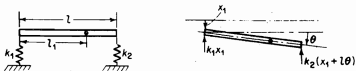
FIGURE 5.3.4. Coordinates leading to static and dynamic coupling.
