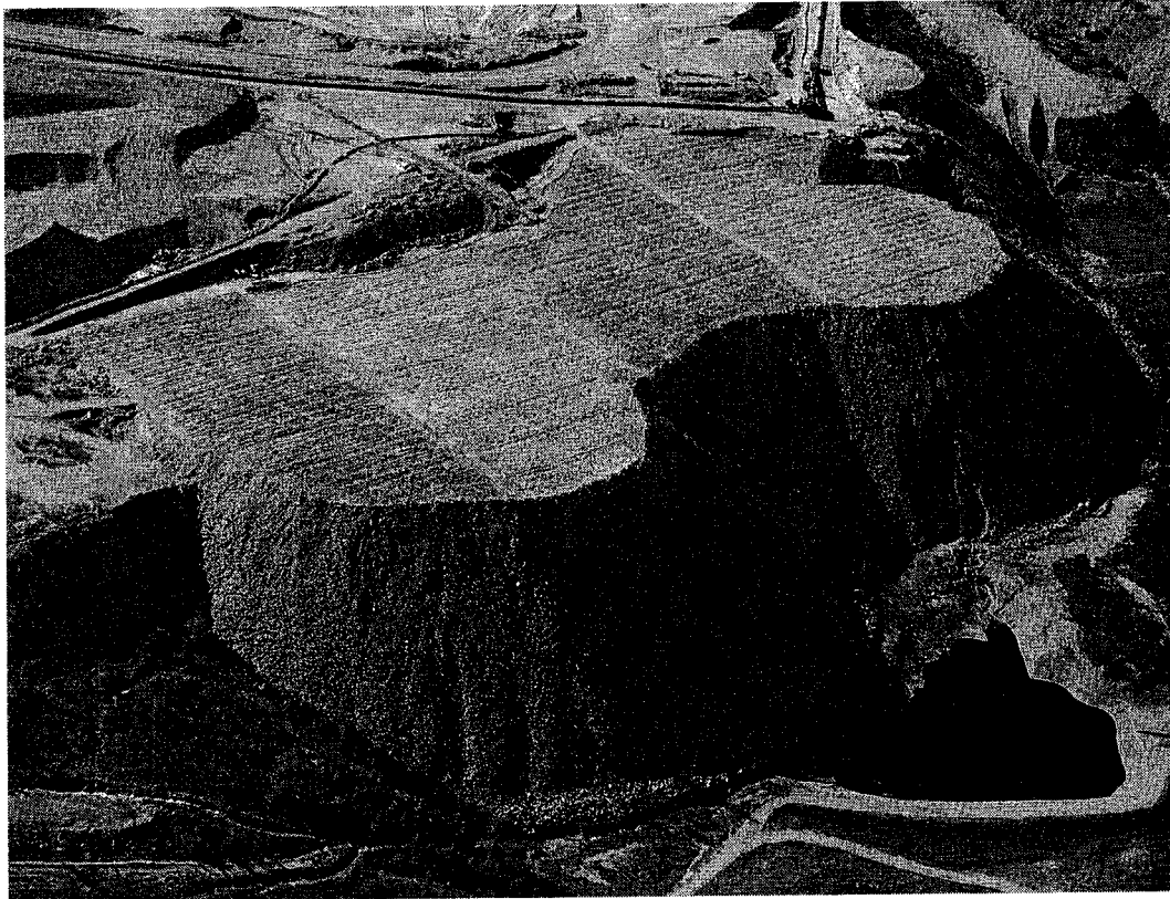
Figure 6.9: A dump leaching operation.
