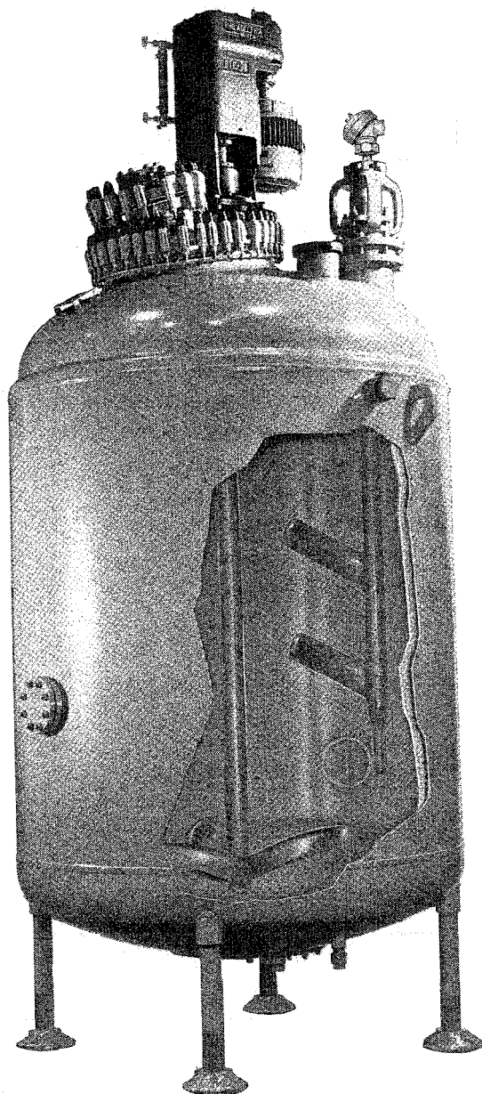
Figure 6.17: Mechanically agitated leaching reactor with heating jacket.
