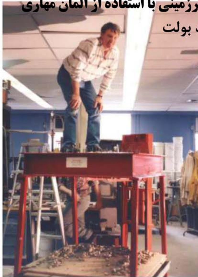
(d) The load-carrying capacity of the bolted gravel plate.
