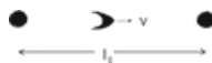
Fig. 1.13 The Lorentz-FitzGerald contraction of the distance between two stars seen by the inertial observer O' in a spaceship
