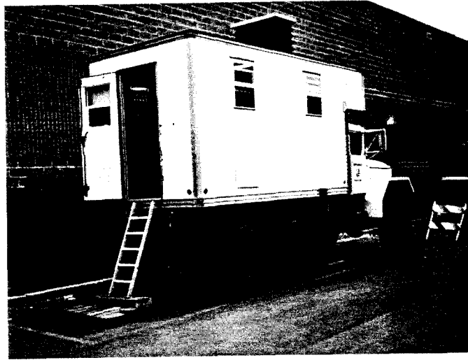
Figure 4.13 A truck-mounted CPT rig. A hydraulic ram, located inside the truck, pushes the cone into the ground using the weight of the truck as a reaction.
