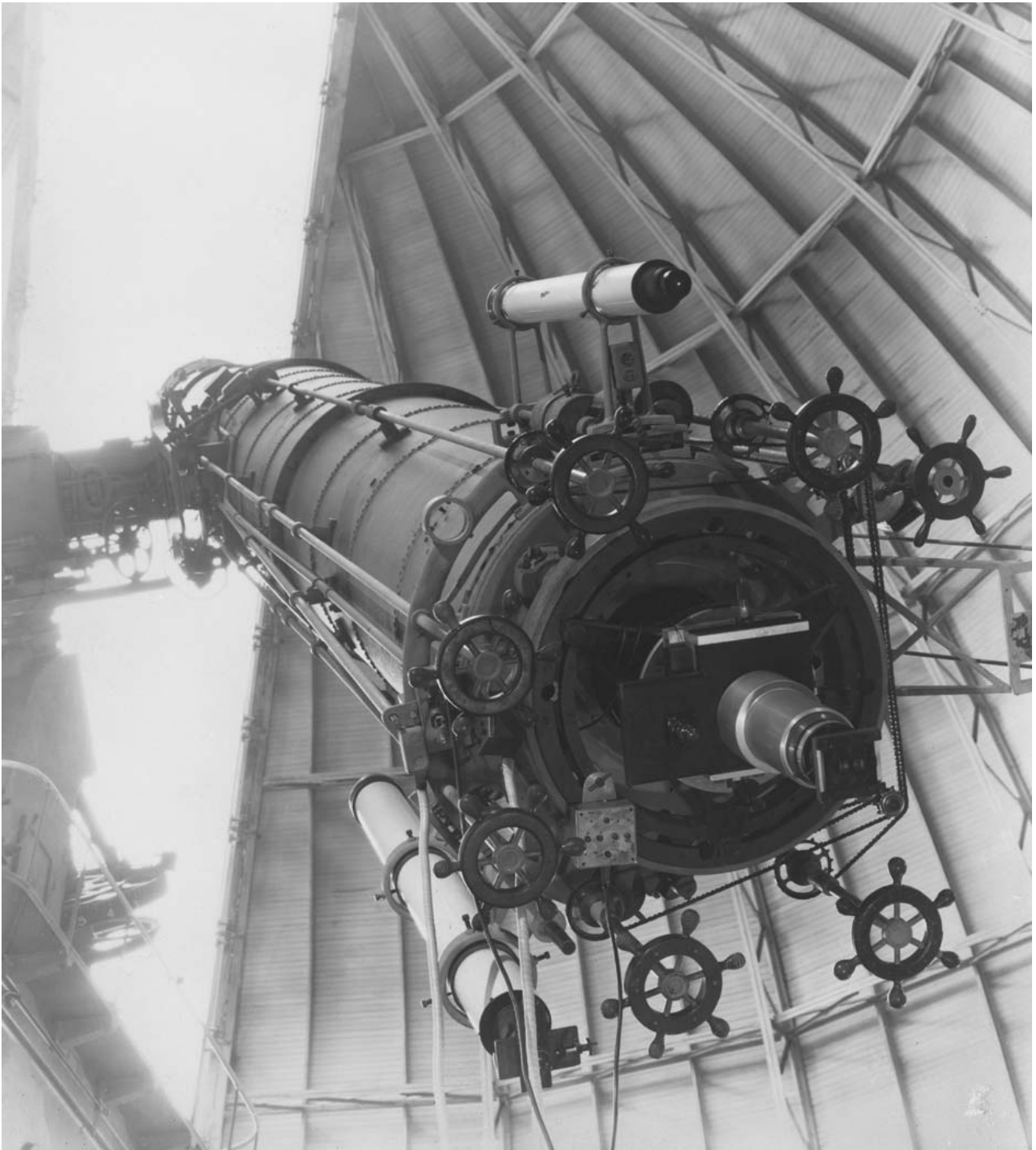
Fig. 3.10. The largest refractor in the world is at the Yerkes Observatory, University of Chicago. It has an objective lens with a diameter of 102 cm. (Photo by Yerkes Observatory)
