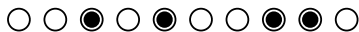
Fig. 1.3 Ten atoms which can accommodate four quanta of energy. An atom with a single quantum of energy is shown as a filled circle, otherwise it is shown as an empty circle. One configuration is shown here.
