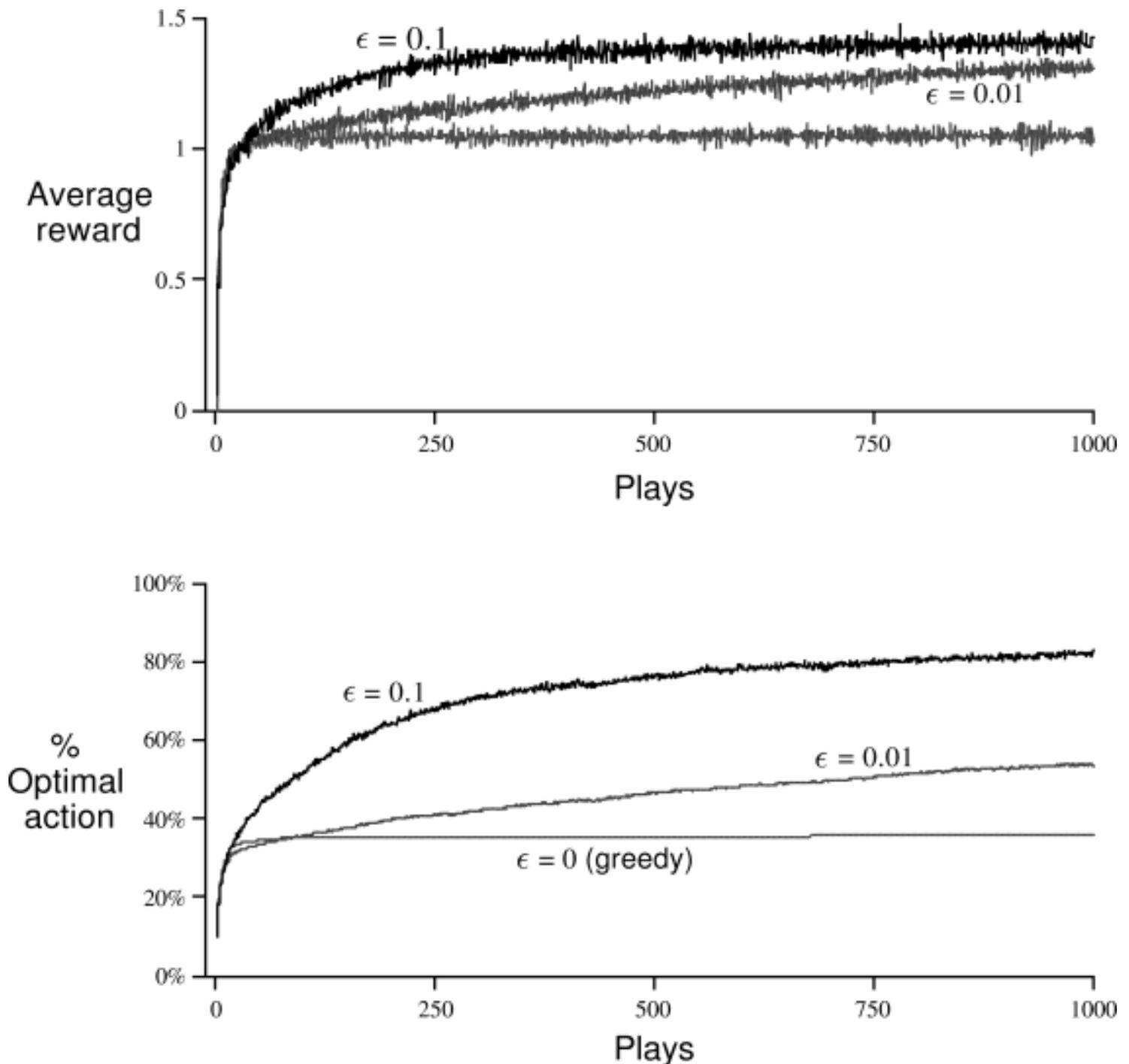
**Figure 2.1:** Average performance of  $\epsilon$ -greedy action-value methods on the 10-armed testbed. These data are averages over 2000 tasks. All methods used sample averages as their action-value estimates.
