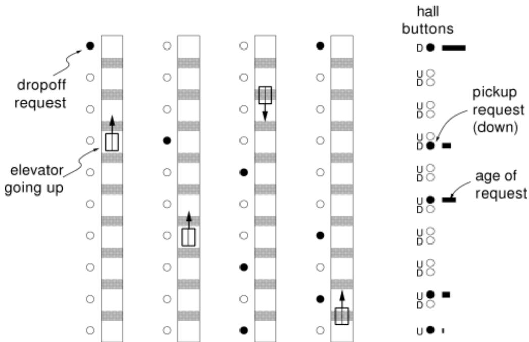
**Figure 11.8:** Four elevators in a ten-story building.
