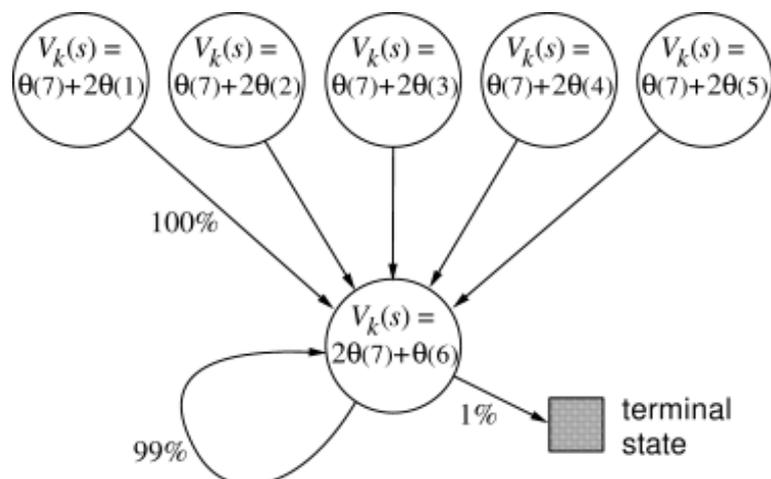
**Figure 8.12:** Baird's counterexample. The approximate value function for this Markov process is of the form shown by the linear expressions inside each state. The reward is always zero.
