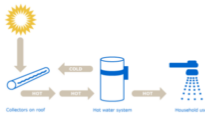
How a Solar Hot Water system works
