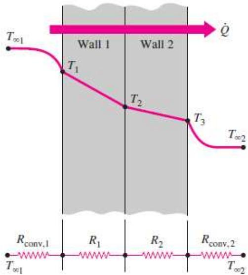
$$\begin{aligned} R_{\text{total}} &= R_{\text{conv},1} + R_{\text{wall},1} + R_{\text{wall},2} + R_{\text{conv},2} \\ &= \frac{1}{h_1 A} + \frac{L_1}{k_1 A} + \frac{L_2}{k_2 A} + \frac{1}{h_2 A} \end{aligned}$$
