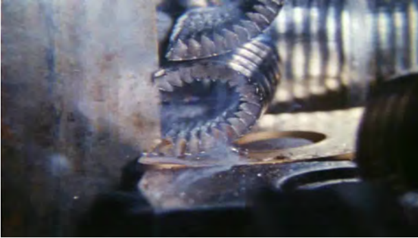
Typical chip breaking sequences with high speed imaging.
